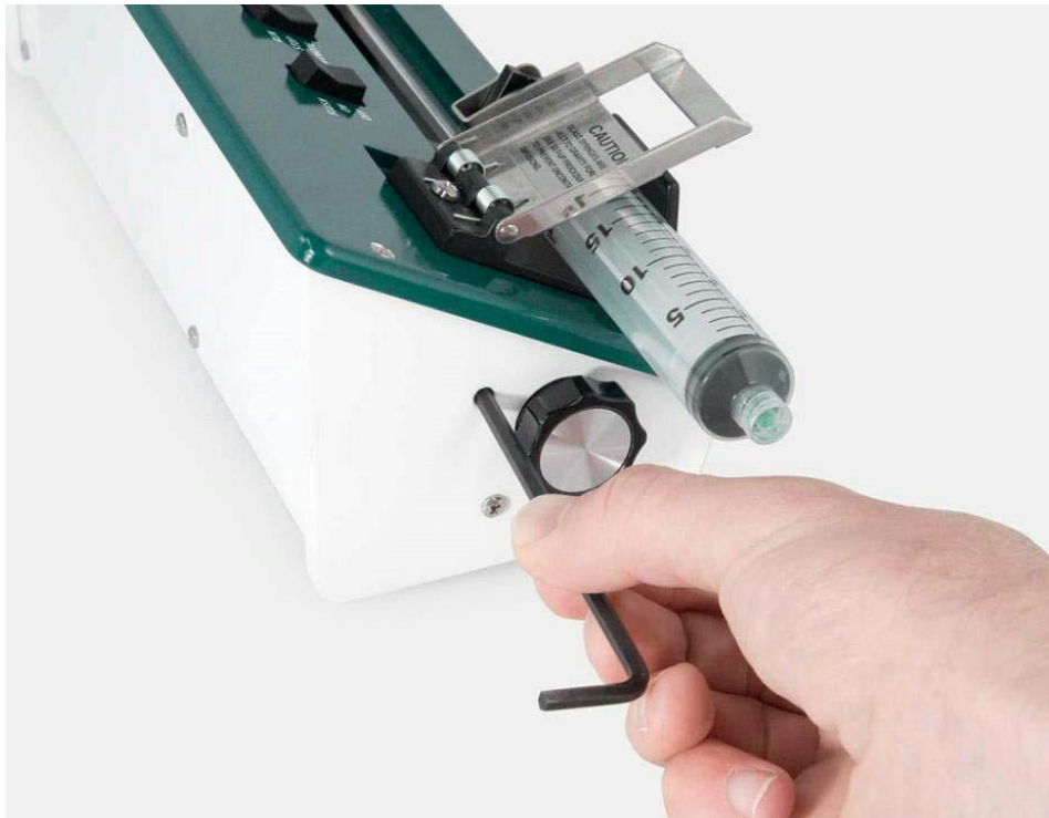
Figure 3.1 - Automatic Shut-off Switch Adjustment
